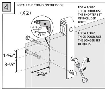
With proper installation, the maximum recommended weight for doors is 200 pounds.
